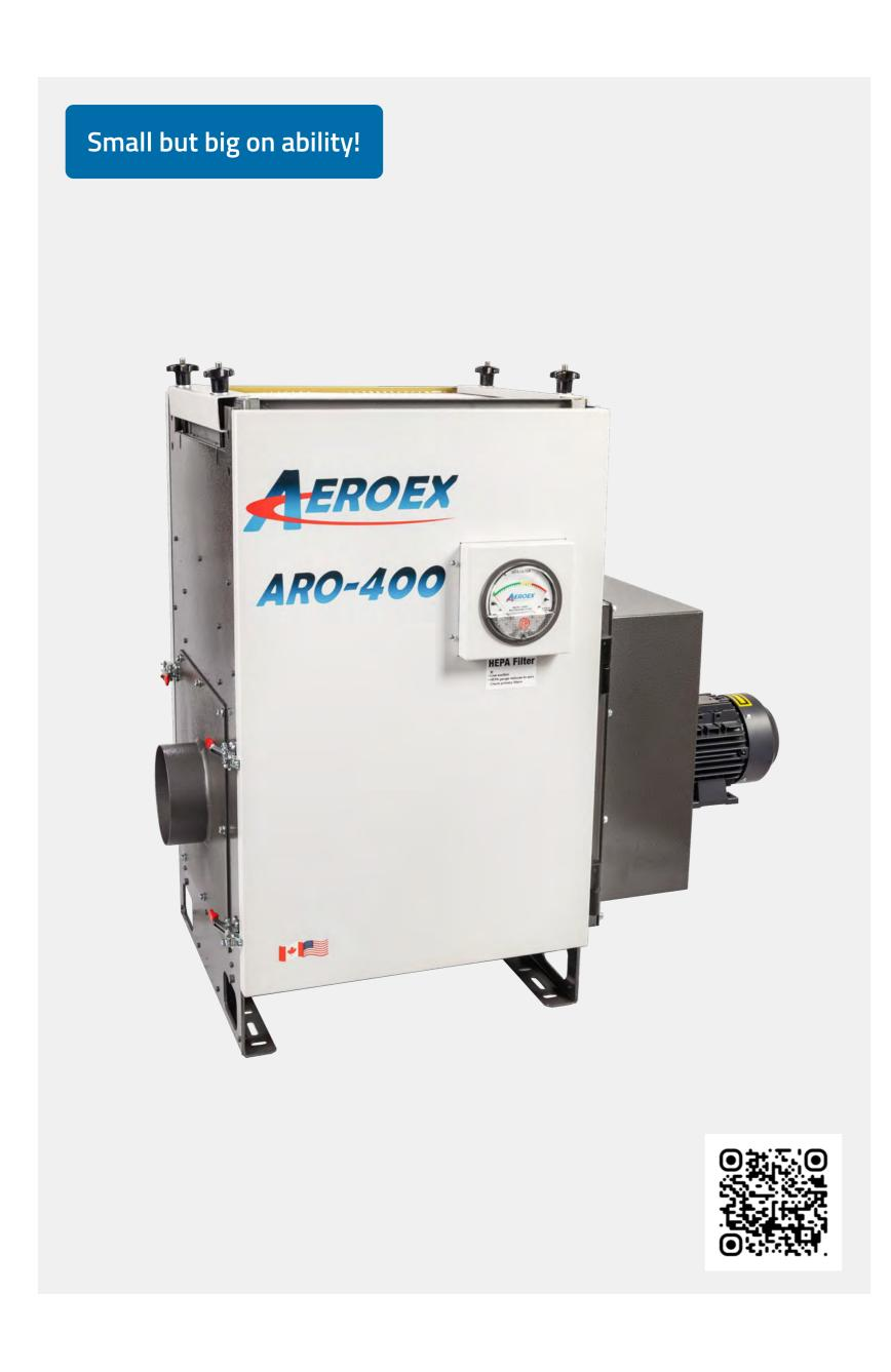
The ARO-400 Mist Collector by Aeroex Technologies is designed for industrial machining and manufacturing environments. Featuring advanced multi-stage filtration with depth-loading fibrebed filters, it ensures prolonged filter life and seamless 24/7 operation.
