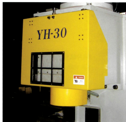
※ 增加安全護罩 with safety cover.
