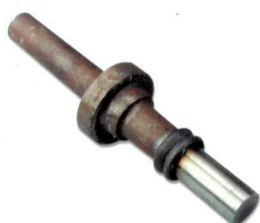
摩擦熔接後的水泵。 Water pump shaft after friction welding.
