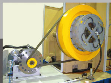
Fast and positive operation by air clutch and brake control. 大扭力直接啟動分離式空氣離合器
