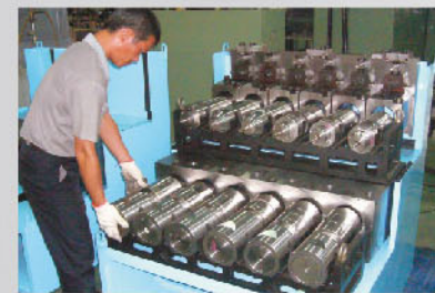
Extra set of die and punch block allows operators to set up another job while machine is running. (Optional) 公母模外吊機構可供快速安裝模具以節省換規格時間 (選配)
