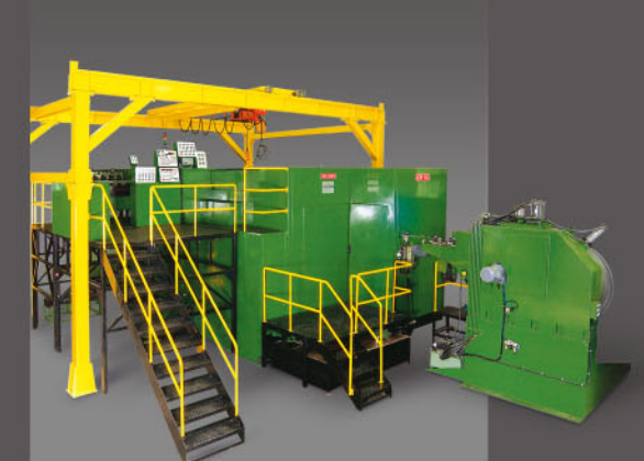
5 / 6 / 7 Station Parts Former
