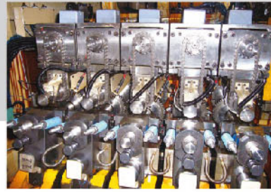
Motorized / digital K.O. length adjustment saves operators a lot of tooling change-over time. (Optional) 人機數位化後通模內長度調整 (選配)
