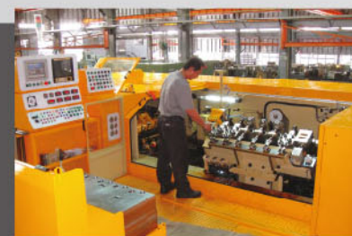
New technical transfer system, Transfer housing lift and turn system, allows operators set up the transfer easily. (Optional) 新型夾仔台90度旋出外調機構 (選配)
