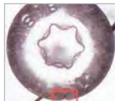
頭上裂痕 Head Crack
